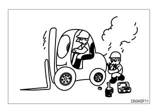
· Unless you have special instructions to the contrary, maintenance should always be carried out with the engine stopped. If maintenance is carried out with the engine running, there must be two men present: one sitting in the operator's seat and the other one performing the maintenance. In such a case, never touch any moving part.
